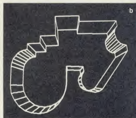
Figure 4. Constructing a 3D solid around a contour: a) input data; b) the object generated by the program
